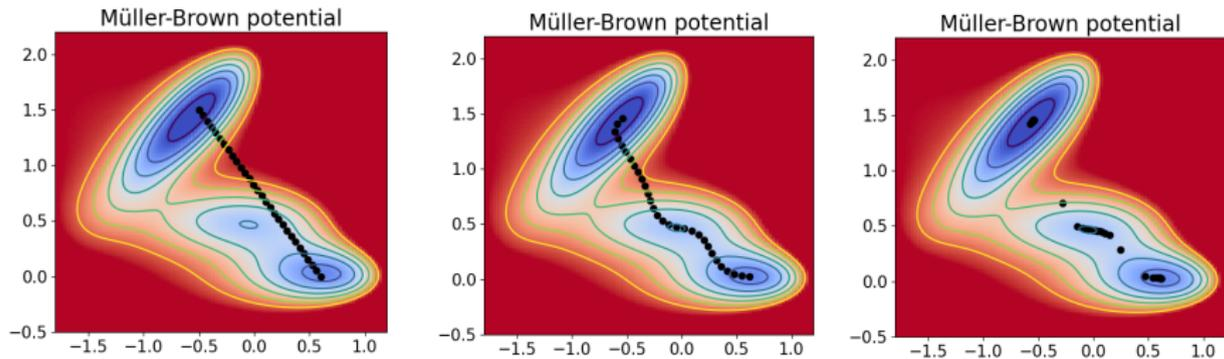
**Figure:** Left: init path. Middle: path after 30 iterations. Right: path after 30 iterations without reparametrization.
